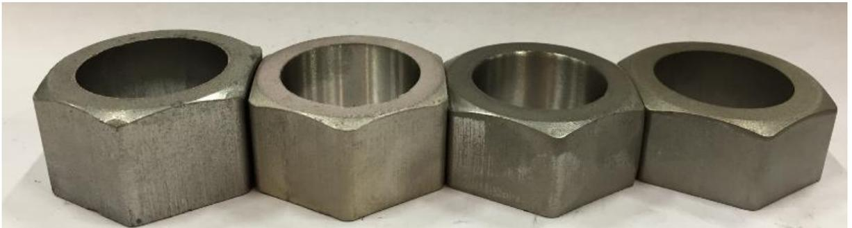
Fig. 3 The four steps in the Scanpac process. Observe the big reduction from step 2 to step 3 Densities from left to right is 84 %, 89%, 97% and finally 99.8% of T.D.
