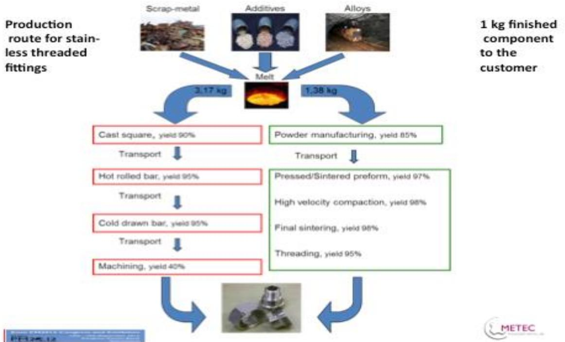
Fig.6 Comparison between the forged route and Scanpac route for production of fittings
