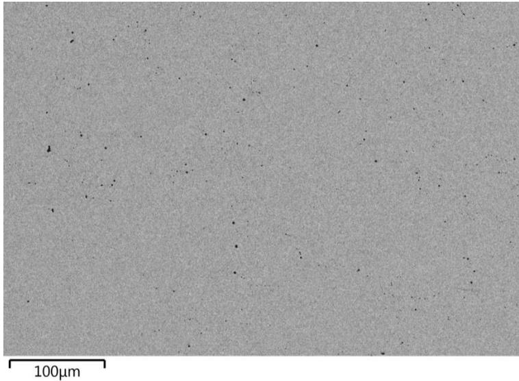
**Figure 3. Micrograph of HIPed sample. Tiny oxides, less than 1  $\mu\text{m}$  in size, are shown in black.**
