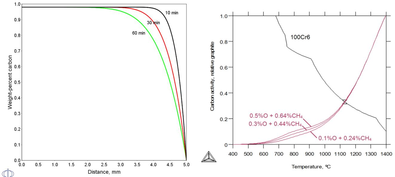
**Figure 5. a) Decarburisation profiles simulated at 1100°C after 10 minutes, 30 minutes, and 60 minutes. b) Carbon activity in 100Cr6 and three different atmospheres with carbon control.**
