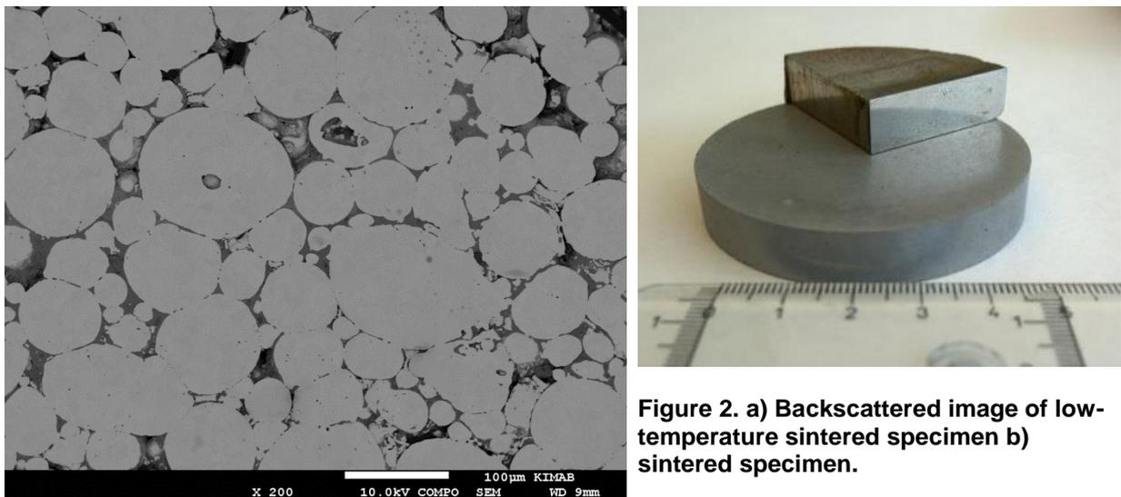
**Figure 2. a) Backscattered image of low-temperature sintered specimen b) sintered specimen.**
