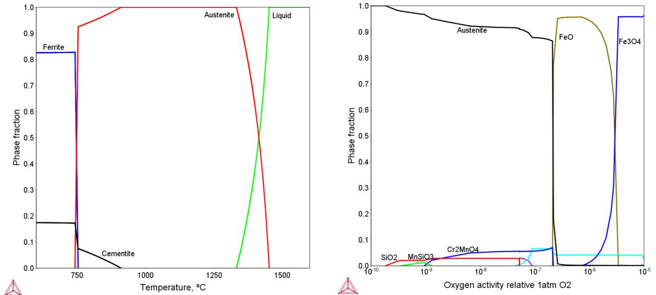
**Figure 1. Equilibrium calculation for Fe-0.98C-0.5Si-0.4Mn-1.5Cr-0.2Co using TCFE7 database. a) Stable phases as function of temperature b) Stable oxides as function of oxygen activity at  $1100^\circ\text{C}$**
